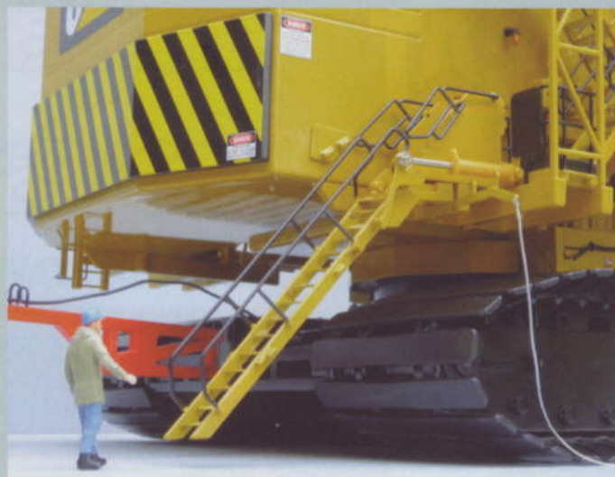
The Caterpillar 7495 with the access stairs lowered.
