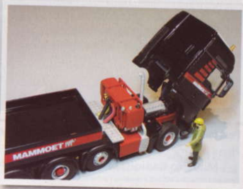
Above: Tilting cab reveals a detailed engine. Left: The MAN TGX.
