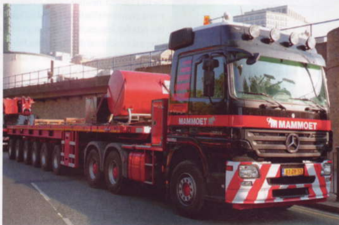
above A real ballast carrier operated by Dutch hauliers Mammoet, as seen on site near the Canary Wharf complex, London.
