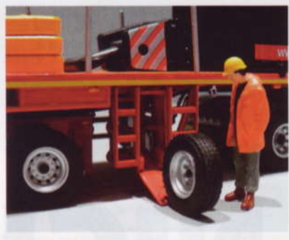
above A really good feature on the Nootboom ballast carrier is the removable spare wheel.
