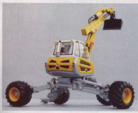
Above: The Menzi Muck A91 excavator and its unusual wheel arrangement.
