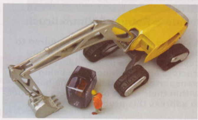
Above: A detachable cab allows remote control working.
