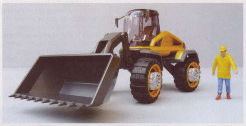
Above: The Gryphin stands high on fully independent suspension.
