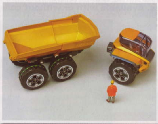
Above: The Centaur has a detachable front axle.
