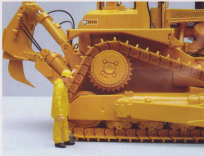
Above: - The excellent detail on the high-drive sprocket.
