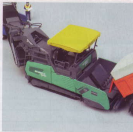
The PowerFeeder receiving asphalt and feeding a paver.
