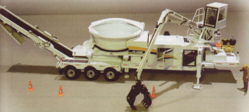
Below: The tub grinder set-up with a few cones marking a safety zone.
