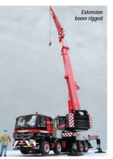
The five stage telescopic boom is metal and the base section has a metal spool, a pair of lights and supports for the boom extension. The boom sections lock into place when extended, and as the extension is pinned to the main boom side it does not fall off when the boom is raised.
