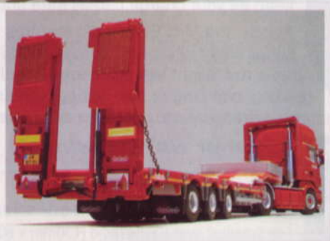
Above: The three-axle Nootboom OSDS trailer. Below: The smaller trailer loaded with Haulotte access equipment.
