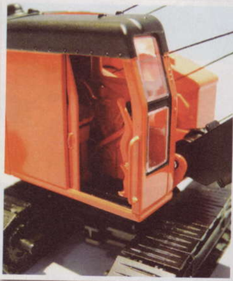
Above: The sliding cab door on the Northwest 25-D shovel. Left: The Northwest 25-D shovel.
