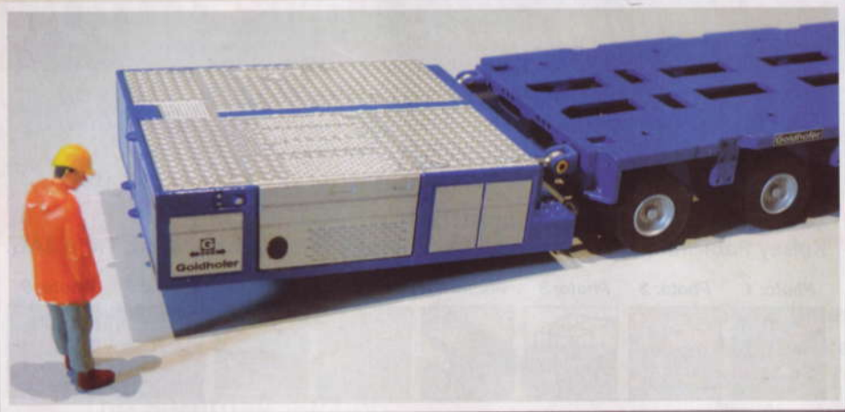
Above: The Goldhofer power pack fixed to the modular trailer.
