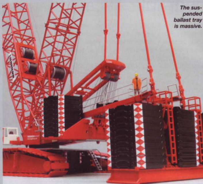
A 300-tonne capacity hook rigged on the main boom.
