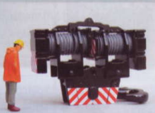
The huge 600-tonne capacity hook.
