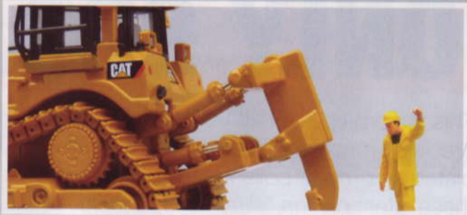
The single shank ripper on the D8T.
